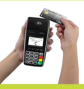
On the back of every card, you'll find a magnetic stripe. It contains the cardholder's name, card account number, and expiration date, as well as special security information designed to help detect counterfeit cards. When the magnetic stripe is swiped through the terminal, this information is electronically read and relayed to the card issuer, who then uses it as crucial input for the authorization decision.
